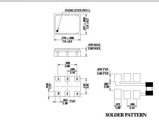
\*0.01µF external by-pass filter is recommended as shown on solder pattern.
