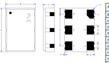
Gold 11.8 µinches 0.3 µm minimum over Nickel 50 to 350 µinches 1.27 to 8.89 µm
