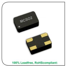
**DIMENSIONS** Recommended Solder Pad: Package: Bottom view 5.00 16 3 1.6 2.35 2 2 pin 1 E/D 1.6 3.20 pin 2 GND 3 pin 3 Fout pin 4 Vdd All dimensions in mm typical
